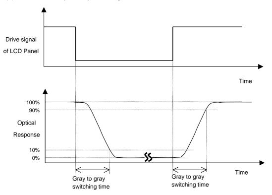
The driving signal means the signal of gray level 0, 63, 127, 191, 255.
